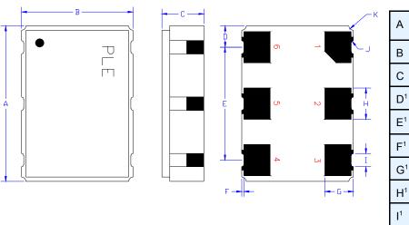
Contacts: Gold 11.8 µinches 0.3 µm minimum over Nickel 50 to 350 µinches 1.27 to 8.89 µm
